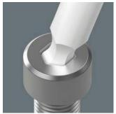
We questioned the classic L-key design, since all too often the screw head recess is rounded out, meaning screws can no longer be tightened or loosen and so the user finds the L-key slipping out of the recess. Wera Hex-Plus tools have a larger contact surface in the screw head. The notching effects reduced and thereby the deformation of the screws. At the same time, as much as 20 % more torque can be applied.
